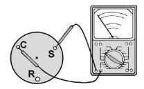
Remove compressor terminal box cover and disconnect wires from terminals. Using an ohmmeter, check continuity across the following:
