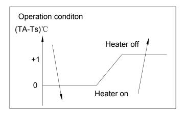
6.7.2.1. When TA < TS, the indoor fan operates firstly, and then the heater operates after 4 seconds.
